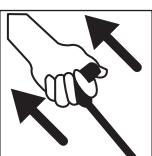
**12****Move the Choke to the OPEN Position**
