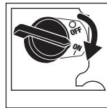
**10****Move the Choke to the CLOSED Position**
