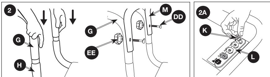
6. Remove colored quick connect nozzles (K) from plastic bag and insert them into correct grommet on the nozzle holder (L). **NOTE:** Nozzles are color coded to match colored nozzles on panel.
