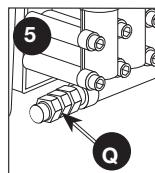
**Detergent Injection System:** Mixes cleaners or cleaning solvents with the water to improve cleaning effectiveness.
