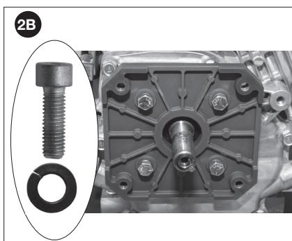
3. Align the key on the engine crankshaft with the key way on the pump (Figure 3A), slide pump onto engine crankshaft, and use a 6 mm hex key to install the four bolts from step one (Figure 3B).
