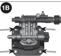
2. Install mounting plate onto engine using 1/2" box wrench to tighten the supplied hex head bolts and split-ring washers. Torque bolts to 15-17 ft-lbs. See Figures 2A and 2B.
